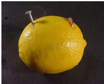
5. Using the alligator clip-ended wires, connect each electrode to one input of the voltmeter, to measure the voltage by the generated battery. Using different electrode materials demonstrates the differences in reduction potentials for various metals.
