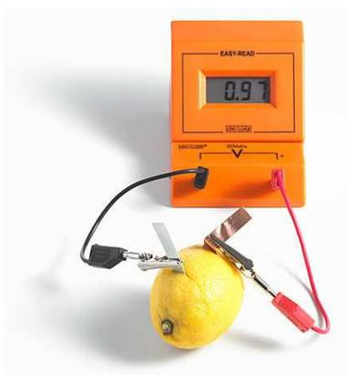
6. A series of cells can be constructed by using multiple lemons (or other food item) and *connecting the cathode on one to the anode on the other*. If enough of the foods are connected together, a voltage large enough to power an electronic device can be produced (e.g., illuminate an LED).
